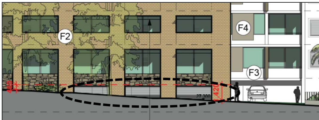
Figure 19: Example of proposed ventilation louvres on the Elizabeth Street frontage of Building B.
